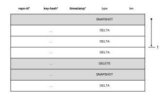
Figure 4: Base+delta chain: Any resource state is reconstructed from the latest non-delta cset prior to the requested t and subsequent deltas.
